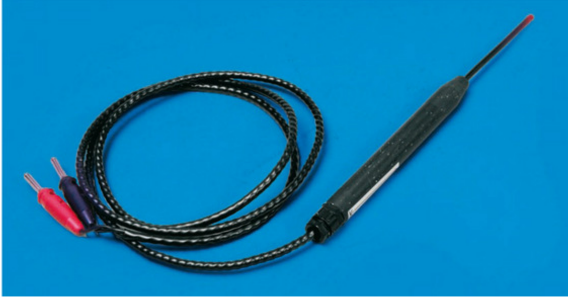
Figure 2.11 – Potential coil probe, Walker LDJ Scientific model PM/S83 (Walker LDJ Scientific, 2013)
