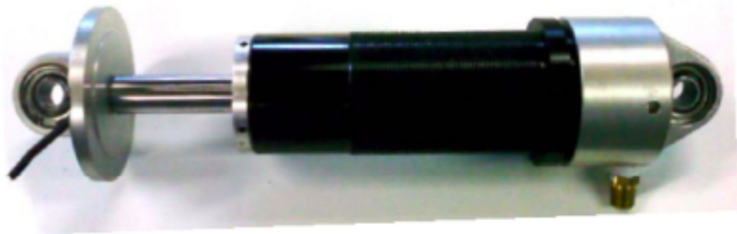
Figure 1.4 - Linear stroke flow mode MREA
